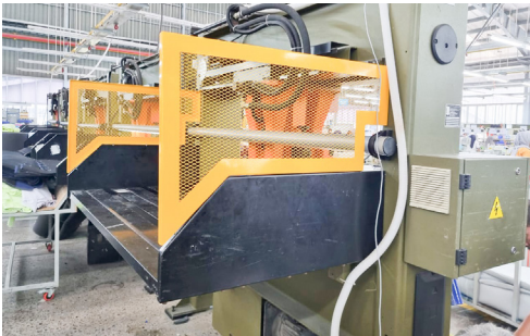
Photo of Completed Improvements to High-Risk Machinery
